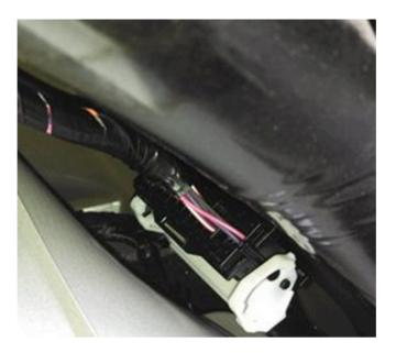
Disconnect X401 and check for corrosion.
