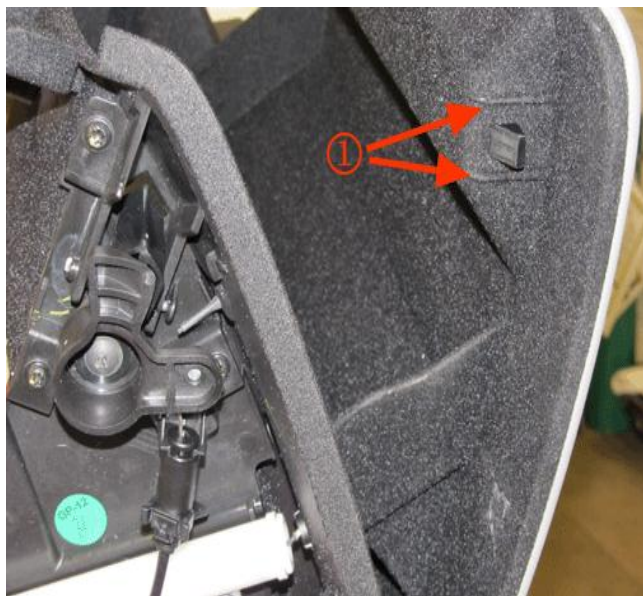
Figure 4- Inboard Ribs Removal
