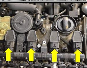
Carefully disengage the locking tab on each ignition coil connector <arrows>.
