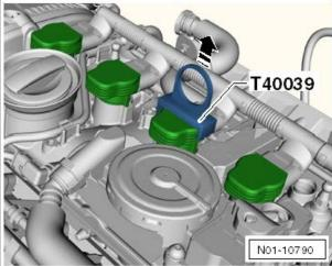
ignition coil approximately 30mm upward.
