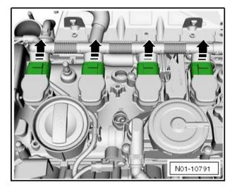
Remove all 4 ignition coil connectors simultaneously <arrows>.
