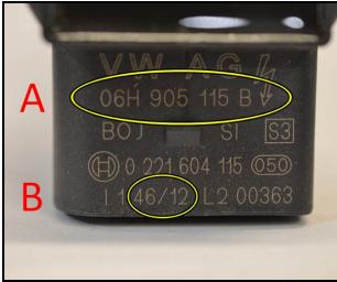
Inspect the part number and build date of all 4 ignition coils.
