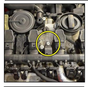
← Remove the T30 torx head mounting screw from the ignition coil wiring harness <circle>.
