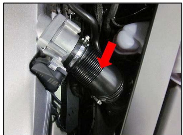
Figure 6. W12 air duct
