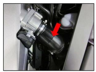
Figure 6. W12 air duct
