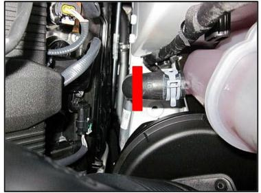
Figure 9. Expansion tank filler hose
