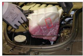
Figure 4. Lifting up coolant expansion tank
