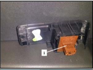
Disconnect connector <1> and remove the handle trim.
