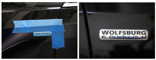
**Step 3:** Remove protective film from adhesive strip. Install badge and evenly apply 15lbs of pressure to seat the tape.
