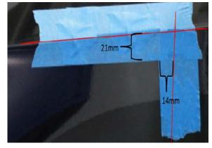
**Step 2:** Measure 21mm down from fender line shown above. Measure 14mm from fender/ door edge. Use easy release tape to mark off the area.
