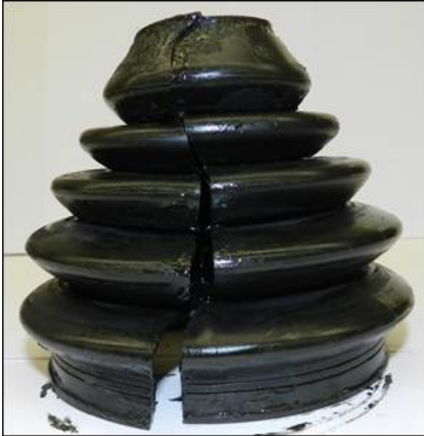
CV Boots should not be cut or sliced upon removal.
