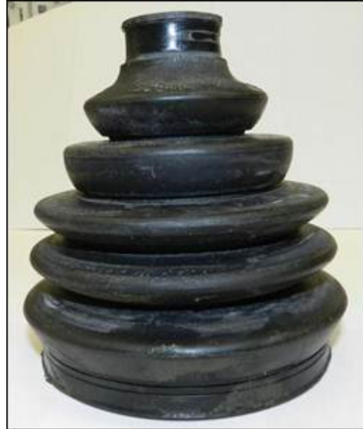
CV Boots should slide off the driveshaft after the removal of the CV Joint.
