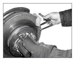
Re-measure brake disc thickness in 4 locations using either the Pro Cut disc thickness measuring tool Part No. 50-902 or the Hunter disc thickness measuring tool Part No. 25-99-2, to verify that minimum thickness is still exceeded. If recorded brake disc measurement is less than the minimum thickness, the brake disc MUST be replaced.
