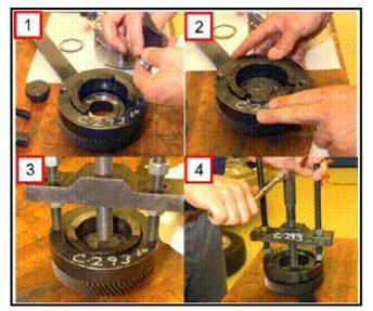
• Using press puller P/N C-293-PA , Adaptors P/N 9738 and a press plug P/N 9678, remove compounder transfer gear bearing cone.
