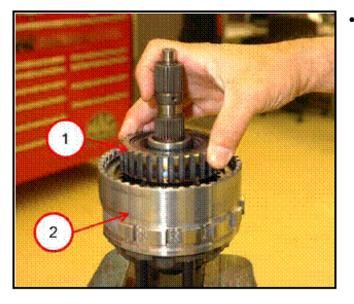
Install overrunning clutch (1) into low clutch (2).
