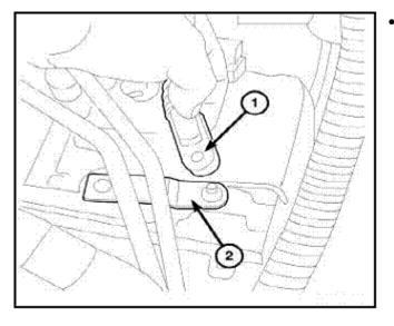
• Remove shift cable (1) from manual valve lever (2).
