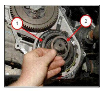
• Make sure select fit shim (2) is located on the transfer shaft (1) prior to installing the transfer gear.
