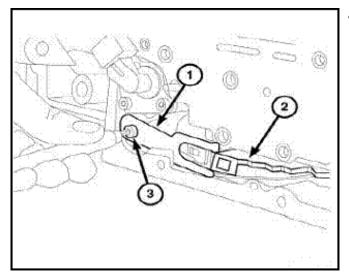
• Remove the screw (3) at the detent arm (1) and remove arm.
