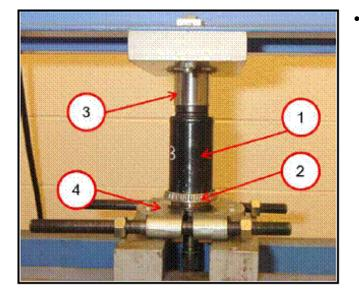
• Using installer P/N 6756 and a press, install the transfer bearing Part. No. 7B0323415 onto the transfer shaft.
