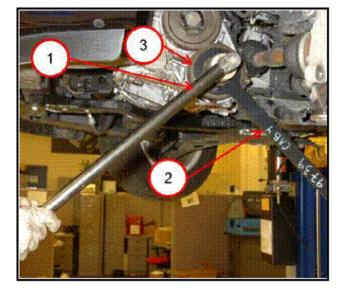
Install the gear holder (2) P/N 9739 onto the transfer gear (3) (underdrive compounder side) and remove the nut.
