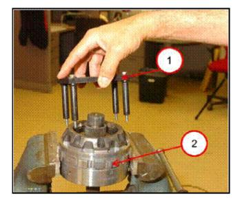
• Carefully clamp the underdrive compounder low clutch (2) into a soft jaw vise.
