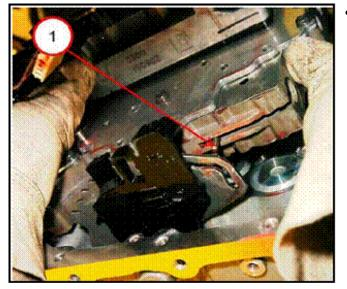
• Lift up on the valve body to clear the manual valve pin (1) past the slot in the rooster comb.
