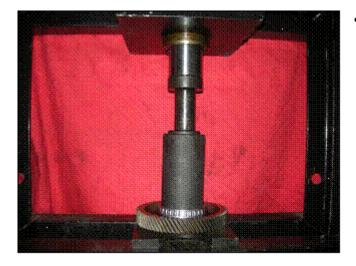
Install the transfer gear bearing cone Part No. 7B0323415 using installer Part No. 6756.
