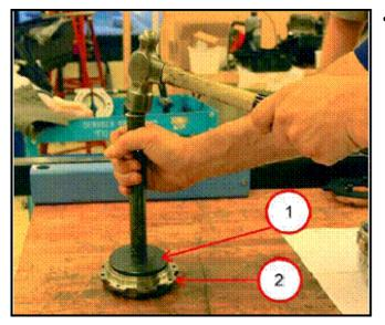
Install the new bearing <u>inner</u> race into the transfer shaft bearing retainer (2) using Bearing Race Installer 9952 and Handle C4171 (1).
