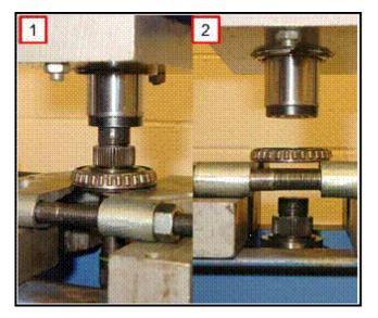
• Using a bearing splitter P/N 1130 (VW Tool 15/3) and a press, remove the transfer shaft bearing.
