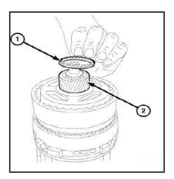
• If necessary, install the helical shim (1).
