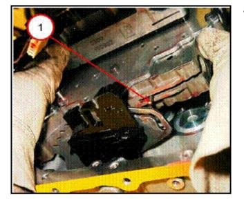
• Position the valve body near the underdrive compounder oil transfer tubes and slide the valve body manual valve pin (1) into the slot in the rooster comb.
