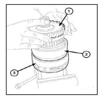
Install the planetary gear (1) set/output hub onto the direct clutch (2).
