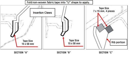
• For section C, the material must be doubled (2 layers thick) to achieve the required thickness as shown in the photo below.
