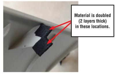
• Once all the non-woven material pieces are in place, re-install the "A" pillar trim using a **NEW** tether clip.
