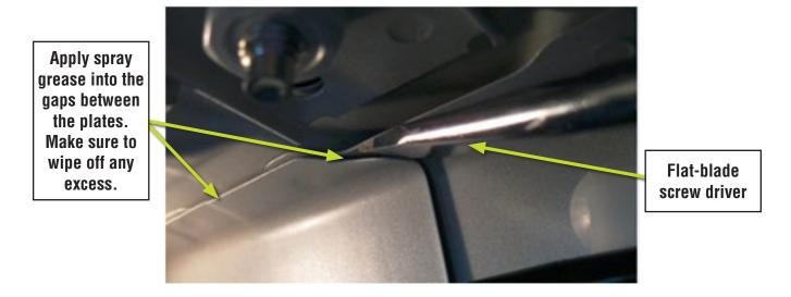
After spraying the grease into the gaps, use a suitable method to **CAREFULLY** reduce the gap between the lower and middle plates as shown in the photo on the next page. Take proper precaution to prevent damage to the paint.
