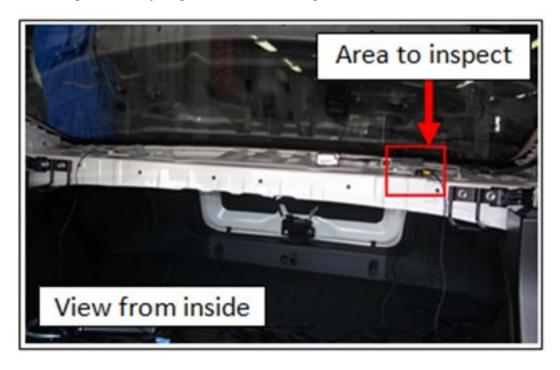
**IMPORTANT:** Due to the tight confines of the package shelf area, use extra caution to protect the rear window glass from damage.
