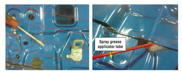
Using the tip of a flat-blade screwdriver, **CAREFULLY** separate the plates of the area approximately 1/8" (3.5mm) as shown in the photo above (left). Do not spread the plates apart any further than necessary to allow the spray grease to be applied as shown in photo above (right).
