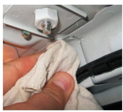
Once the gap has been reduced, wipe off any excess grease then be sure to touch up any damage to the finish as necessary. Once the Case #1 procedure has been completed, road test the car to confirm the sound no longer exists. If the sound persists, the following Case #2 procedure will be required.
