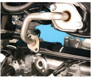
• There is no need to remove the oil dipstick tube or the original oil filter from the front chain cover. While the cover is removed, store it face (front side) down to minimize the chances of damaging the machined sealing surface on the block / head side. Also, don't use it as a tray to store other removed parts. This will help to reduce the chances of contamination entering the various oil passages throughout the front cover.
