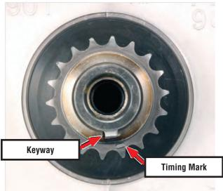
• Arrange the timing marks as shown below, turning the crankshaft **CLOCKWISE** into position. Align the indicator link with the timing mark on the crankshaft sprocket, keyway with the dowel pin.
