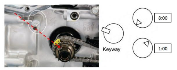
• Align the indicator links to the timing marks found on the outside of the sprocket assemblies as shown in the photos below (Exhaust sprocket face images will vary with / without exhaust VVT).
