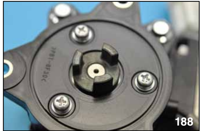
PRG Drive Unit Motor Coupling Gear "Close Up"
