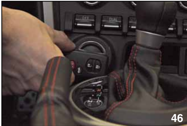
Remote Transmitter Position for Dead Transmitter Battery
