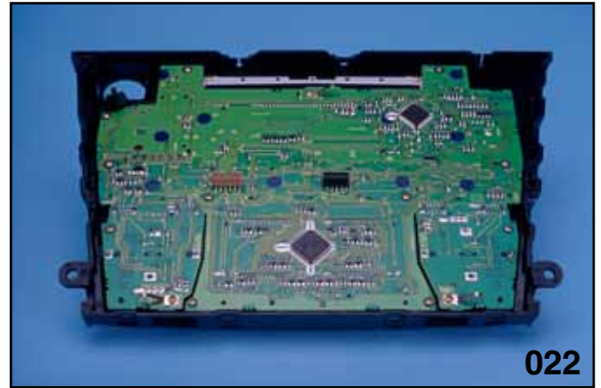
REAR VIEW OF CONTROL PANEL
