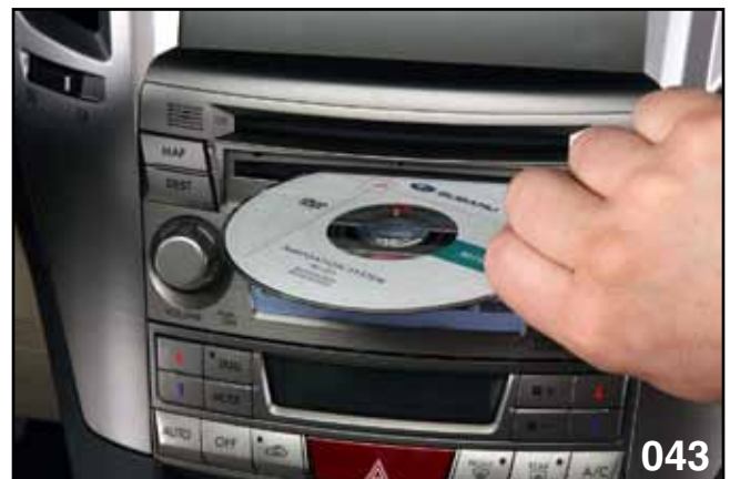
INSTALLING NAVIGATION DVD
