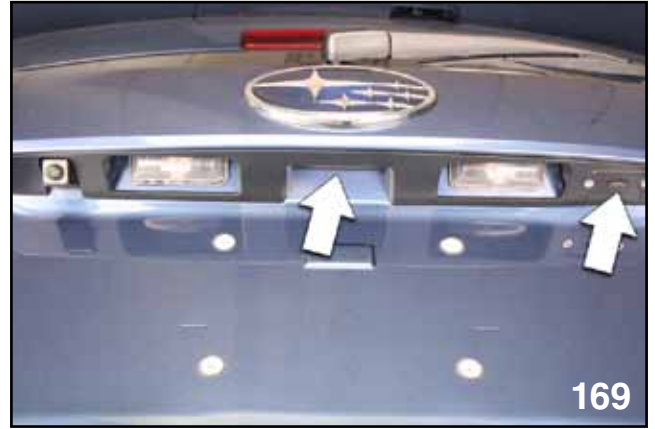
Gate Opener Switch Location & Keyless Access Lock Button
