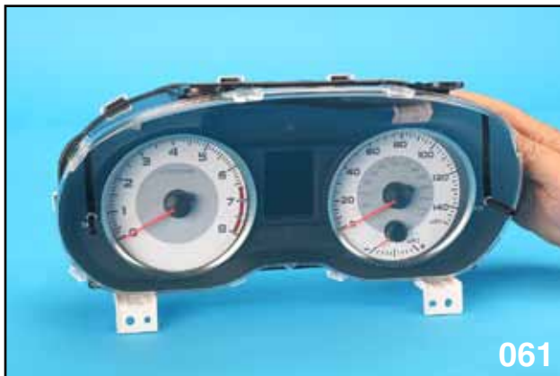
COMBINATION METER FRONT VIEW
