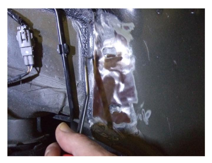
5. Use a 2 x 4 and apply moderate force with a hammer to flatten the outer wheel apron to minimize the clearance to the middle side sill.
