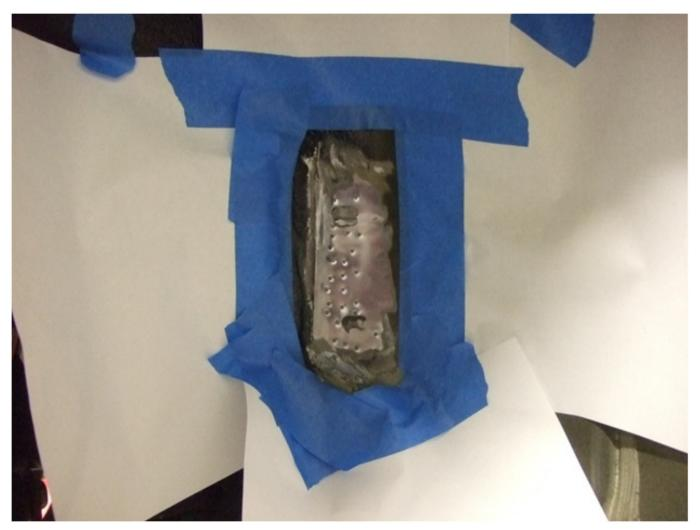
12. Spray the area using etching primer (two coats are recommended). **NOTE:** Make sure to read and follow the cautions and instructions on the can before using. Make sure etching primer is dry before applying second coat and before proceeding to the next step.
