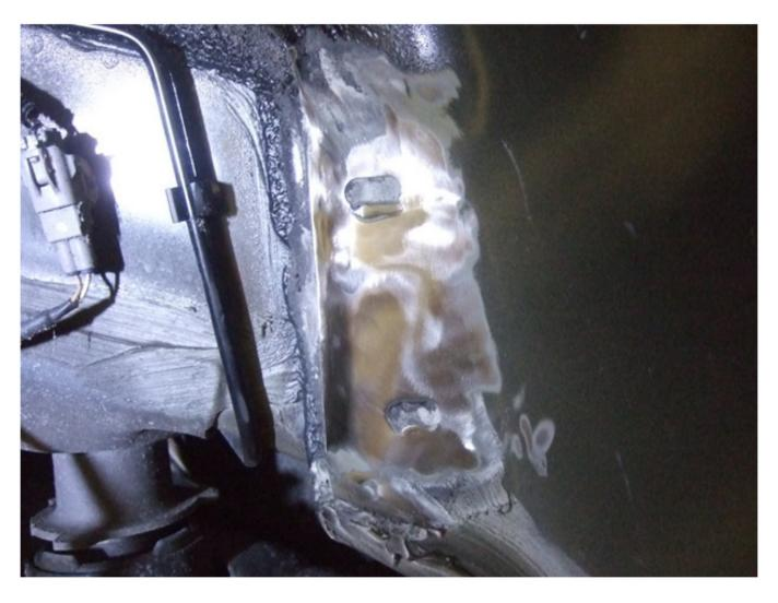
There are 3 layers of sheet metal which are secured together.
