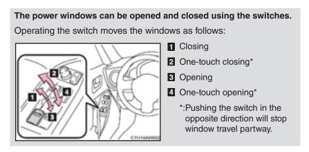
**NOTE:** This power window main switch logic change will in no way effect the prescribed function of the switch. If the customer concern relates strictly to the amount of time required to press the switch to engage the One-touch feature, replacing the switch will have no effect on their concern.
