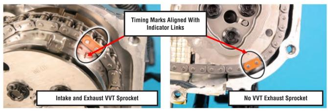
• Install the chain guides and tensioner. Once proper positioning has been confirmed, pull the pin to release the tensioner. With your hand, grab and squeeze the upper and lower chain / guides together as shown in the reference photo below to allow the plunger in the tensioner to fully extend and "click" into its furthest notch.
