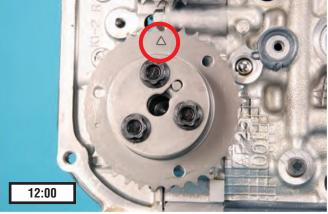
• Align the indicator link with the timing mark on the crankshaft sprocket as shown below.
