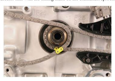
• Same as the left side, align the indicator links to the timing marks found on the cam sprocket assemblies. Install the chain guides and tensioner. Once proper positioning has been confirmed, pull the pin to release the tensioner. With your hand, grab and squeeze the upper and lower left side chain / guides together to allow the plunger in the tensioner to fully extend and click into its furthest notch as shown in the previous (right side) photo.
