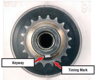
• Arrange the timing marks as shown below, turning the crankshaft **CLOCKWISE** into position. Align the indicator link with the timing mark on the crankshaft sprocket, keyway with the dowel pin.
