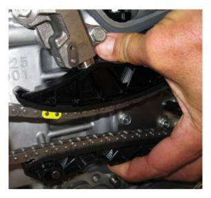
• Rotate the crankshaft COUNTER-CLOCKWISE until the crankshaft sprocket timing mark is at the 6:00 position. Position the cam sprocket timing marks as shown below; intake 6:00, exhaust 12:00.
