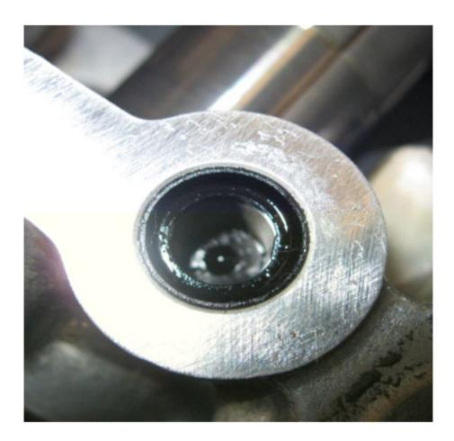
• To begin timing chain re-installation, turn the crankshaft **COUNTER-CLOCKWISE** until the crankshaft sprocket keyway is back to the 6:00 position. NOTE: The keyway is **NOT** a timing mark.
