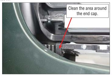
5) Apply sealant under the front of the end cap ensuring that the silicone is filling the gap. **Note:** Make sure nozzle is small enough to apply sealant into the gap.
