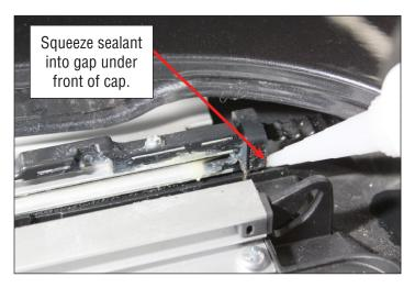
6) Using a right angled pick tool (pictured below) or similar, move a small amount of the sealant around the sides and along the bottom of the end cap and the outer side to ensure the seam is filled.
