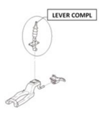
Once the customer's concern has been confirmed to be associated with the shift lever, replace the lever assembly following the service procedure outlined in the applicable Service Manual.
