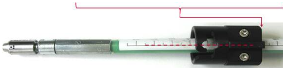
Figure 9: Arrow indicating how the back side of the adaptor must align with the scale. Red dotted line indicating how the longitudinal slot must align with the black line on the scale.
