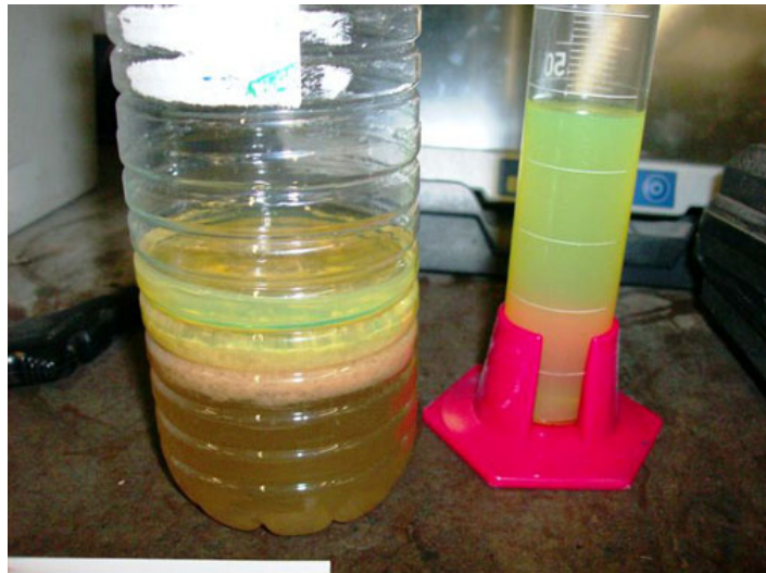
Figure 5. Fuel in the left container is contaminated.
