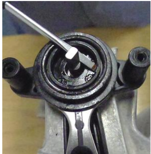
Figure 5. Removing the seal with a screwdriver.
