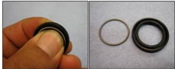
Figure 3. The image on the left shows the correct way to remove the spring. The image on the right shows the spring after it has been removed.
