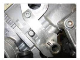
Figure 14. Engine adaptor on bank two.
