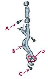
Figure 10. Loosening the coolant tube
