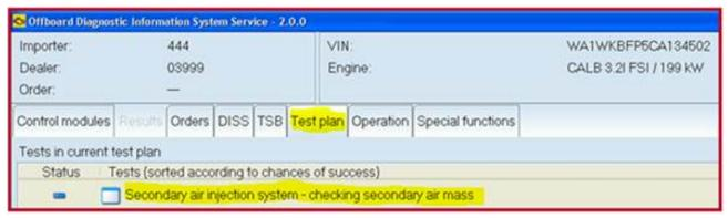
Figure 1. Selecting the test plan in ODIS.
