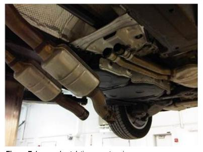
Figure 7. Lowered catalytic converter pipes
