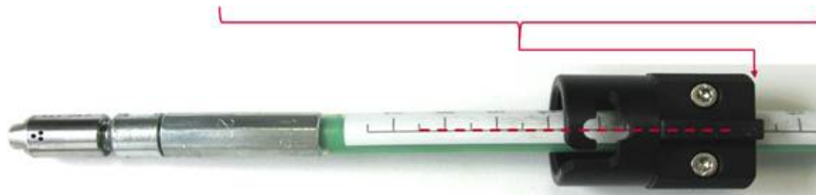
Figure 12: Arrow indicating how the back side of the adaptor must align with the scale. Red dotted line indicating how the longitudinal slot must align with the black line on the scale.
