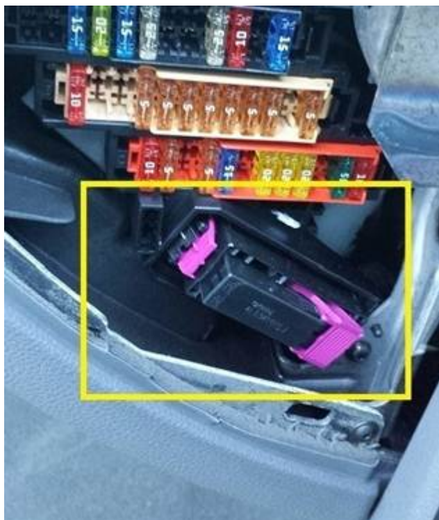
Figure 2. T46b CAN disconnect plug, right dashboard.
