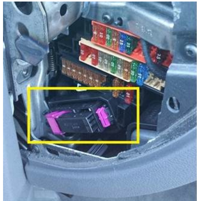
Figure 1. T46a CAN disconnect plug, left dashboard.
