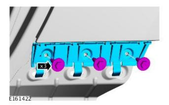
**5.** Remove the rocker panel moulding bracket.
