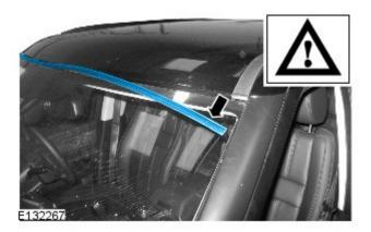
2. NOTE: Ensure no damage has been caused to the upper windshield finisher.
