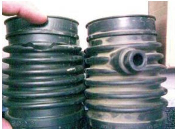
Figure 3. Crack in the intake hose.
