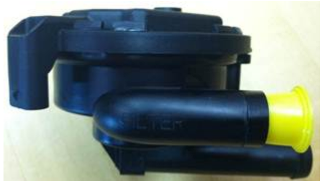
Figure 4. Example of plug inserted inside the pressure sensor filter pipe.
