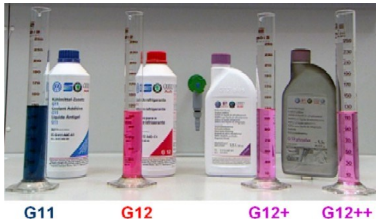
Figure 1. The color of each type of engine coolant. G11 (green-blue), G12 (red), G12+, G12++ and G13 (purple).
