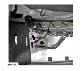
9. A CAUTION: Make sure that the ground cable is fully secured in the area of the luggage compartment lid latch, so that the ground cable cannot come in to contact with the latch.
