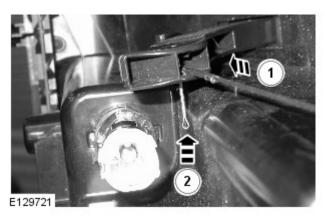
4. Fold the protruding ends of the cotter / split pin.
