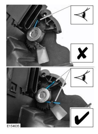
**6.** Install the door latch (see TOPIx Workshop Manual section 501-14: Handles, Locks, Latches and Entry Systems).
