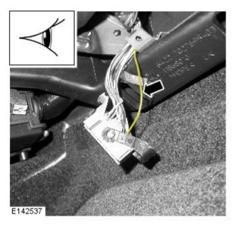
**26.** Using a suitable tool, cut the wire approximately 50mm from the connector.
