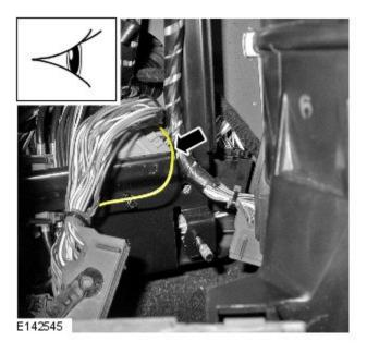
**10.** Using a suitable tool, cut the wire approximately 50mm from the connector.
