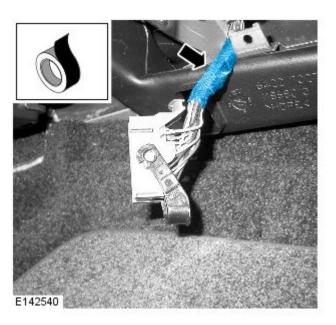
**29.** Using a suitable tie strap, secure the harness to the connector.
