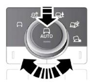
To disengage Automatic ("AUTO") programs, the rotary selector needs to be raised to the elevated position.
