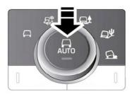
When operating the vehicle in Automatic ("AUTO") program, the vehicle will determine and apply the approriate program for driving style and surfaces.
