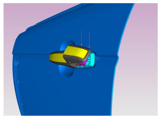
Approach the vehicle with the Door Lock Cover tilted upwards. There is a pair of clipping features that need to be carefully located into the gasket behind.
