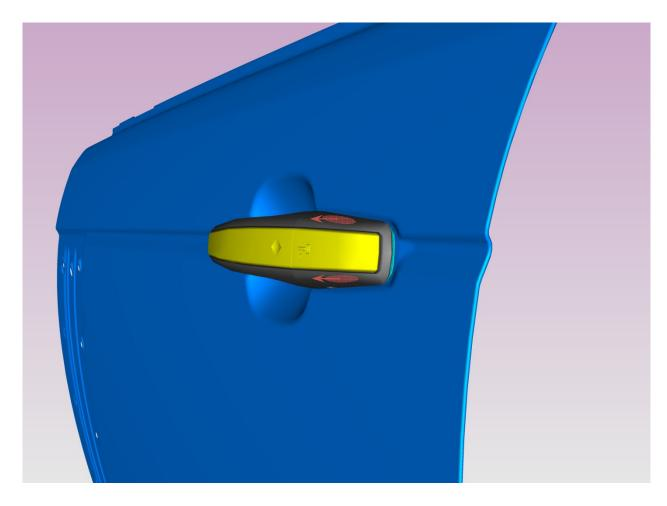
Rotate the Door Lock Cover downwards until a positive click is felt / heard, as the lower retention lug snaps into place in the gasket. Check the Door Lock Cover is secure by gently pulling it, it should remain securely in position on the vehicle.
