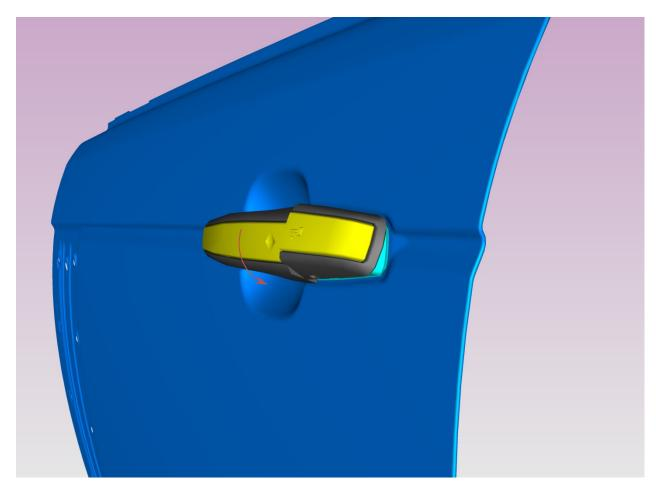
Located both of the clipping features into the gasket in a downwards motion. Once the upper retention lugs are located, rotated the Door Lock Cover downwards to engage the clip on the underside
