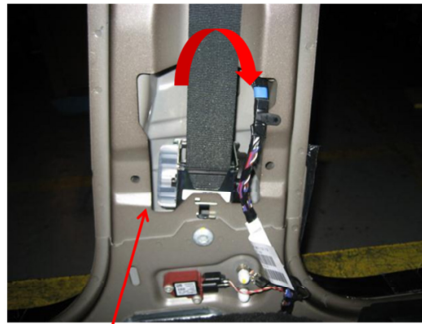
Retractor moved clockwise by the bolt torque, non parallel gap to the B pillar
