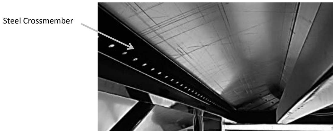
Figure 3: Later unit with a rear steel crossmember
