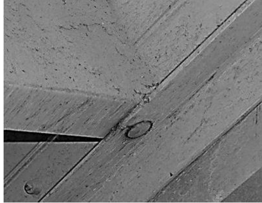
Figure 8: Cracks at side extrusion and Z plate connection.
