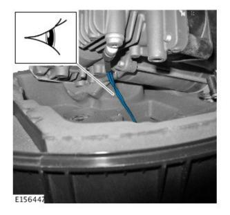
7. NOTE: The protective sleeving must be trimmed to a suitable length on a suitable surface prior to installation. Make sure the protective sleeve covers the entire length of the thermistor harness.
