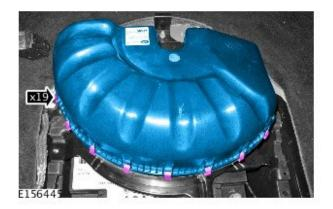
11. Install the two securing bolts (10Nm).
