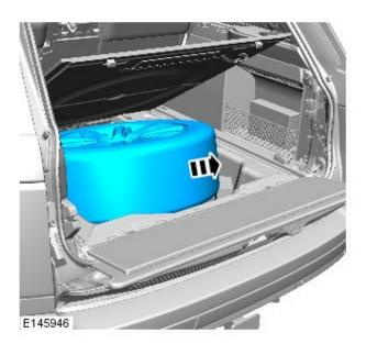
2. NOTE: The air compressor unit is protected by an acoustic box which tilts to allow access to the vehicle battery.
