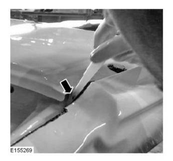
**9.** A dabbing action with a wetted finger is effective for smoothing the sealant into the gaps without a mess.
