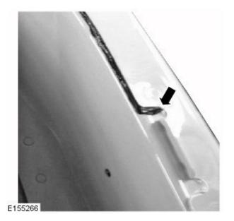
6. NOTE: The area must be clean and dry prior to applying the sealant.
