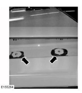
4. NOTE: The area must be clean and dry prior to applying the sealant.
