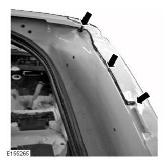
5. NOTE: The area must be clean and dry prior to applying the sealant.
