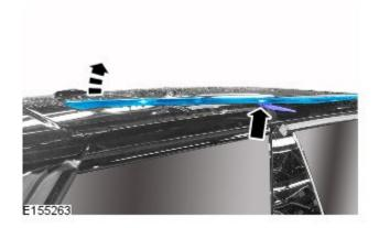
3. NOTE: The area must be clean and dry prior to applying the sealant.
