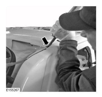
**7.** Make sure the sealant covers the gap at the rear of the roof.
