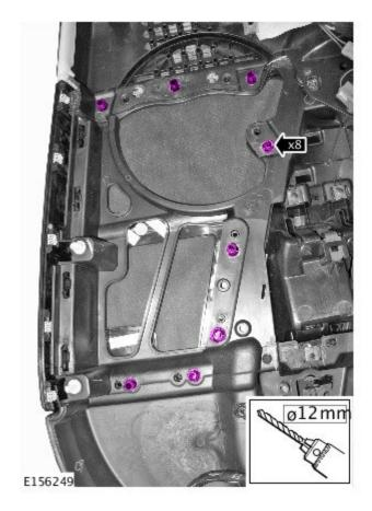
10. NOTE: To avoid surface damage, ensure area is clear from swarf and debris.
