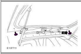
4. Remove the three (3) retaining nuts.
