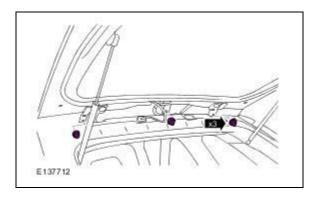
11. Install the two (2) retaining bolts.
