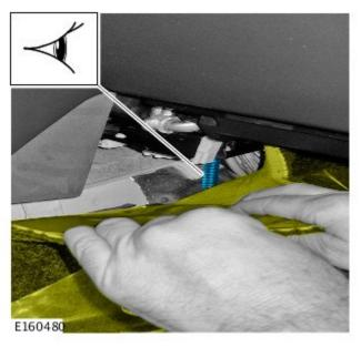
**3.** Check to see if the Climate Control system drain tube is connected correctly.
