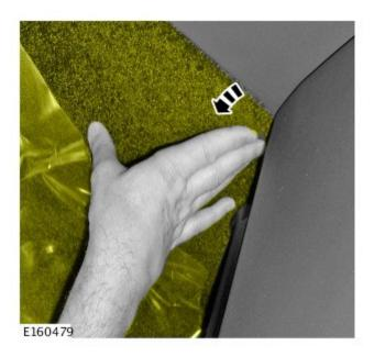
**2.** Pull the carpet down to expose Climate Control system drain tube.
