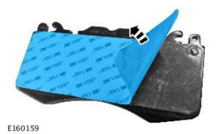
4. NOTE: Do not apply grease to the piston contact area
