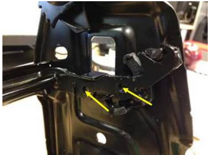
Figure 4. Bracket in incorrect position.
