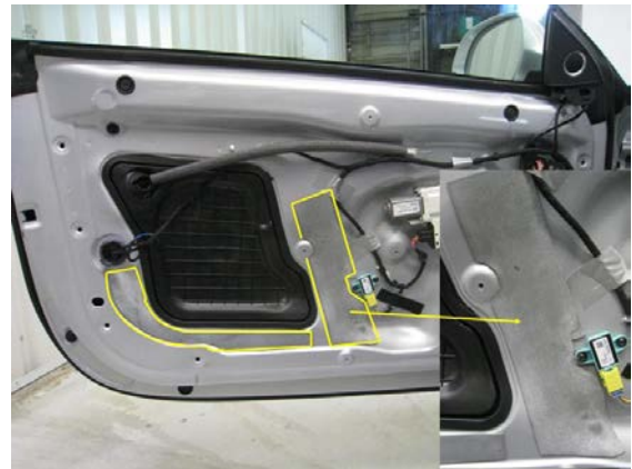
Figure 7. Areas to apply sound absorber.
