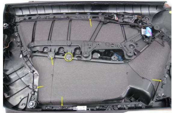
Figure 4. Weld points of the door panel.
