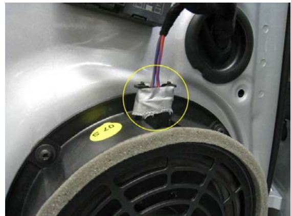
Figure 8. Duct tape surrounding the speaker connector.
