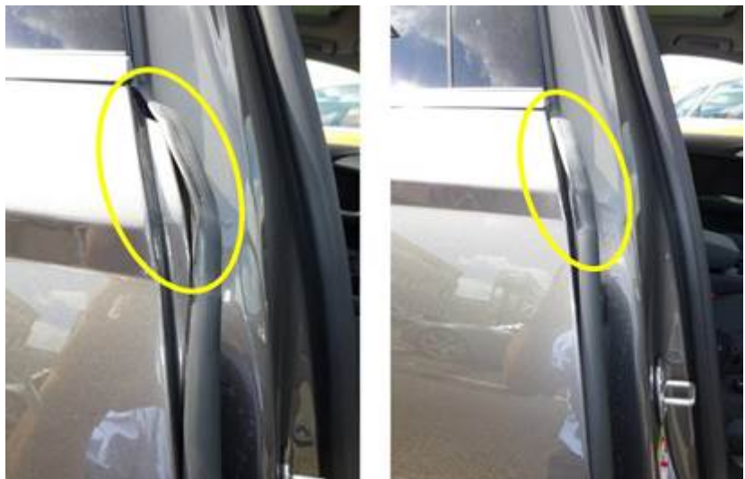
Figure 1. Example of deformed seal on rear door.
