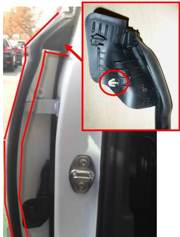
Figure 3. The section of seal to be removed (left) and clipped-in area (inset-right)
