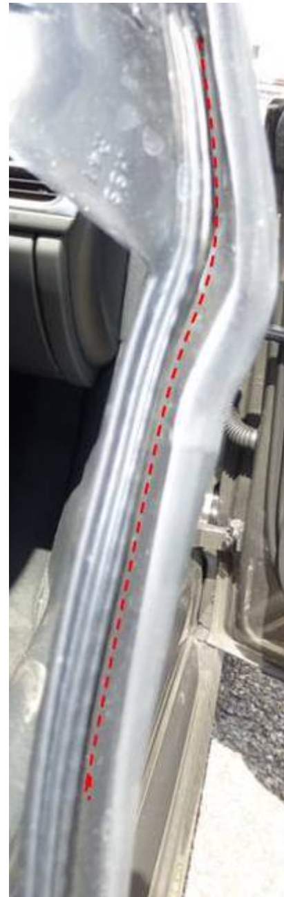
Figure 6. Seal clamping surface; red line indicates where to apply the bonding glue.
