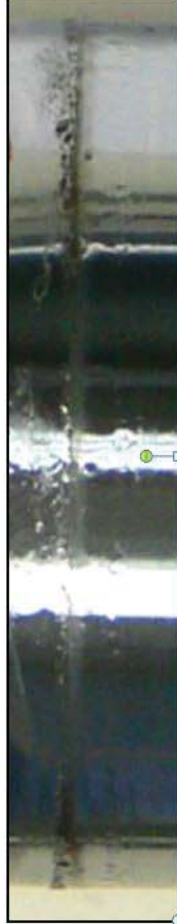
Fig. 4: fixed fork tube with formation of streaks → Shaft seal ring or surface of fixed fork tube damaged
