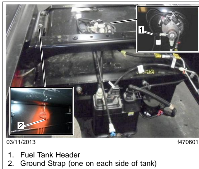
Fig. 1, Fuel Tank Electrical Connections and Hoses
